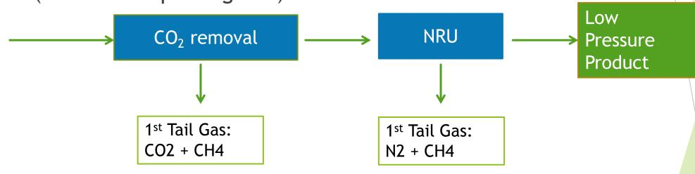
High Energy Consumption (require product compressor and high recycle ratio)
