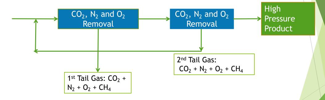
► (4) New Two-step purification: CO<sub>2</sub>, N<sub>2</sub>, O<sub>2</sub> Removal Unit
