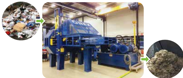
Organics Extrusion Press (OREX) Separates Organics from Mixed Solid Waste to provide feedstock for co-digestion
