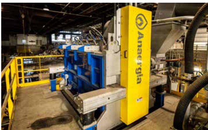
Anaergia’s Organics Polishing System (OPS) Produces a Clean Organic Liquid Slurry for WWTP Digesters.
