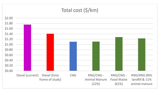
Figure 3: RNG/CNG operational costs at carbon neutrality
